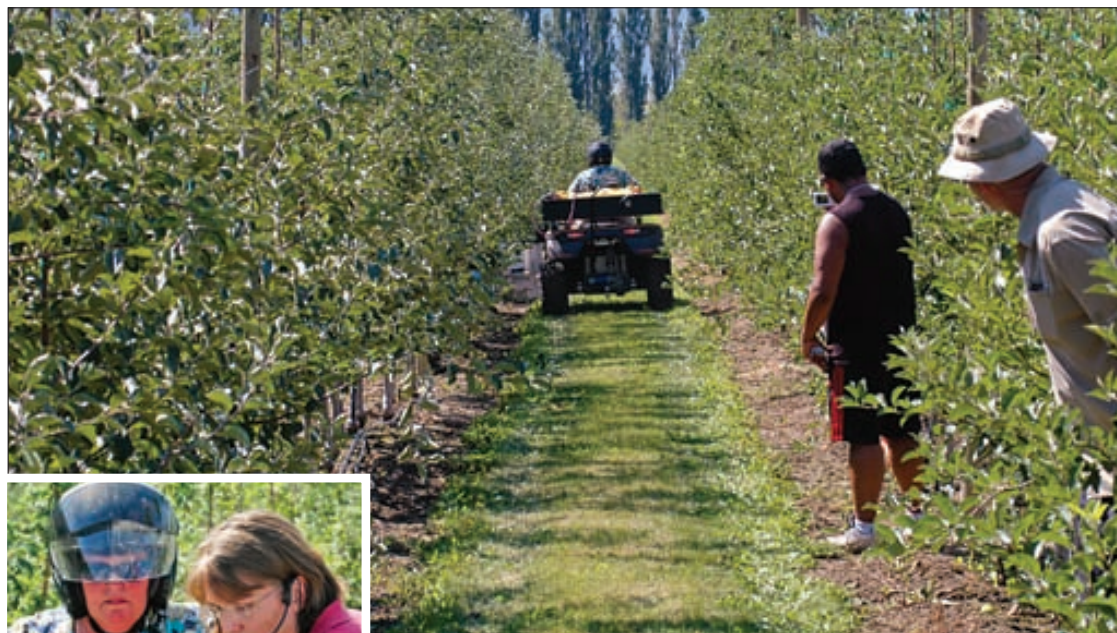
SEEKING WEEDS: An electric vehicle with a WeedSeeker electronic sensing unit, which applies organic herbicides, may save growers money, early research results indicate.
