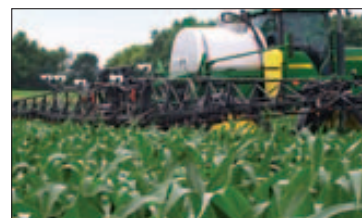
GREEN READER: Greenseeker scanners read the corn leaves' color and vary the N rate to help corn reach the yield goal. Photo: NTech Industries.
