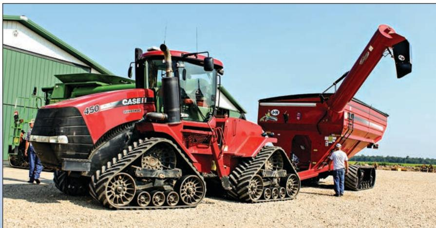
**MUST-HAVES:** Tracks are a necessity for the Rinehart family. In an effort not to disturb the soil, they rely heavily on tracks on their farm equipment.
