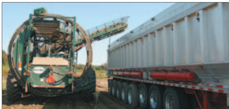
LOAD TIME: After the digger wheels lift the beets out of the ground, the beets are placed on the elevator, which rolls them to the truck. During early harvest of the headlands, Adam Bauer drives the semi in reverse alongside the harvester so he doesn't have to turn around.
