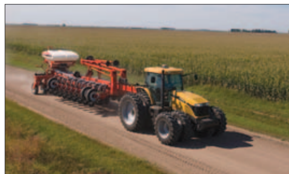
360-DEGREE VIEW: A new feature on the Challenger MT675C is a brand new cab. The four-post cab, surrounded by 67 square feet of glass, is almost 30% larger than the previous model.
