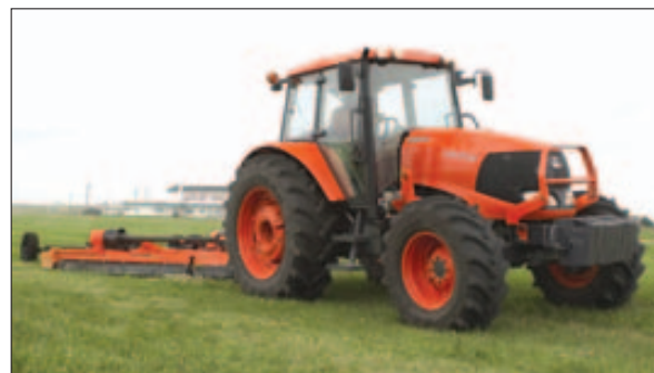
KUBOTA'S NEWEST: The M135X offers electronic-engine system controls, bi-speed turning, electro-hydraulic shuttle shift and a power-shift auto mode with a new central command LCD monitor.
