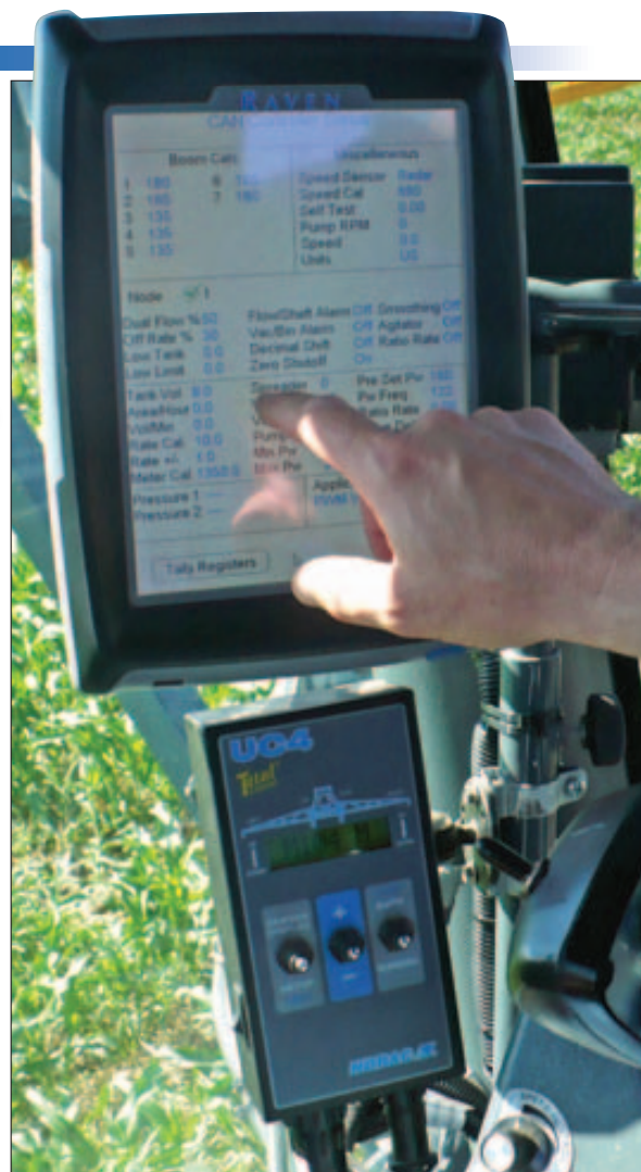
SET THE FLOW: A programming screen allows setup of spray rate, speed and other details for application over an entire field.
