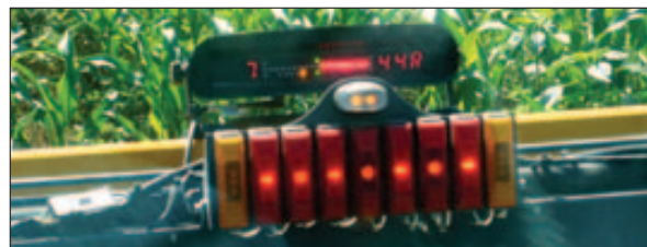
ALL NOZZLES: As each nozzle begins to spray, a light indicates it is operating. If a nozzle clogs or quits, the light for that row goes out.
