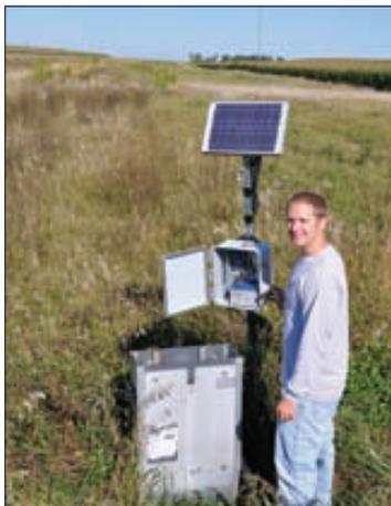
**HARDLY KNOW IT’S THERE:** Keegan Kult checks the automated water-quality monitor at the outflow control structure of a bioreactor on the Van Diest farm. The tops of inflow and outflow water control structures are the only visible traces of working bioreactors.
