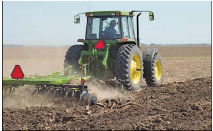
distribute total tractor weight properly between front and rear axles.
