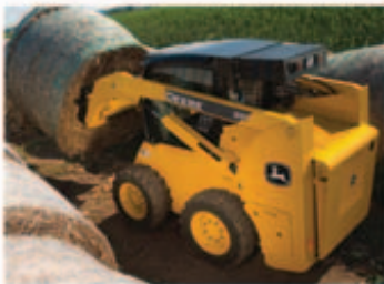
John Deere 313 skids 45 HP, only 59" wide, Tipping load 2,525 pounds, Radial Lift boom
