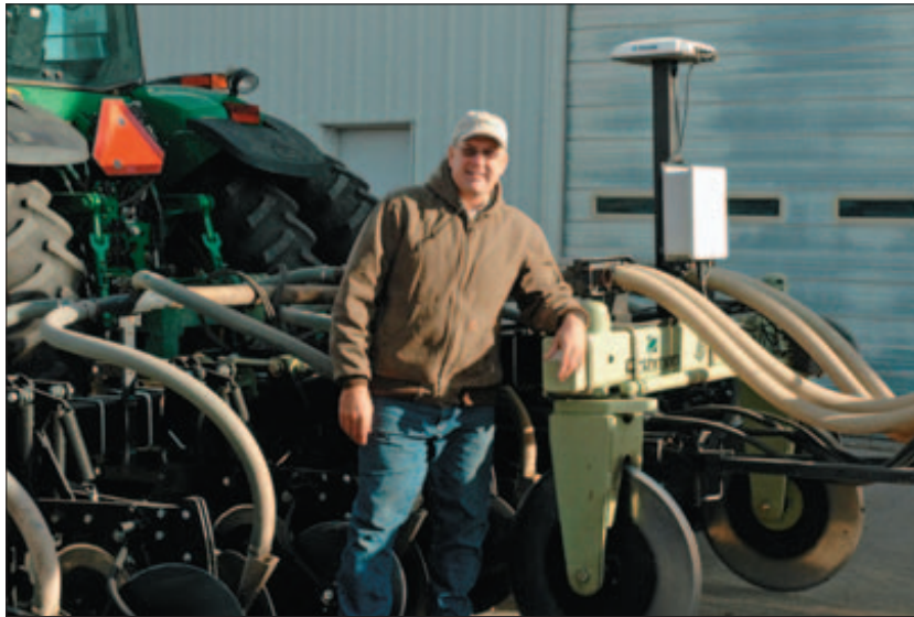
PRECISION PLACEMENT: Don VerMeer uses this implement steering system with his strip-till fertilizer applicator. He uses the same implement steering system on his corn planter.
