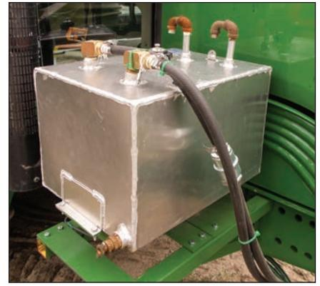
valves connected the auxiliary fuel tank to the tractor's engine.
