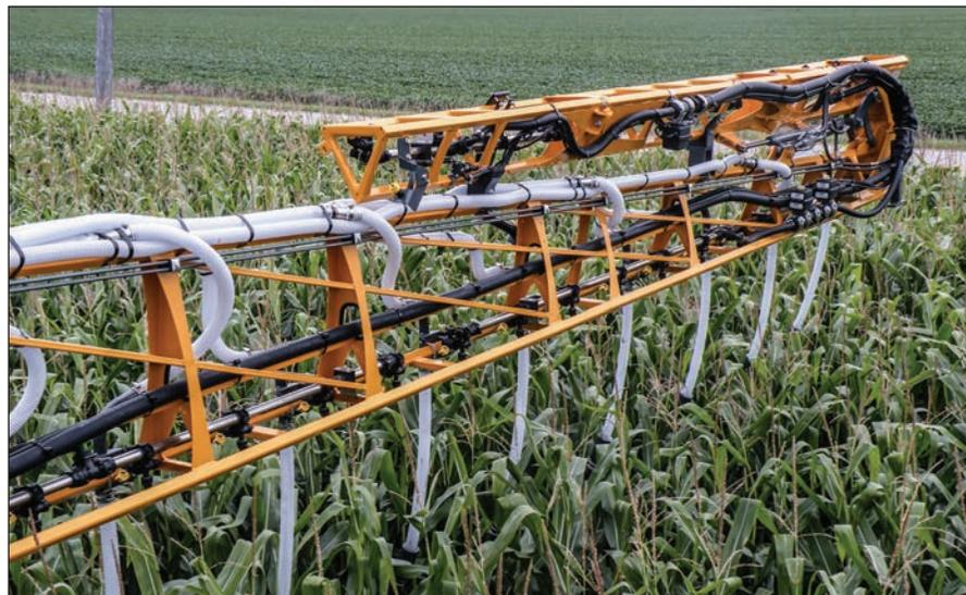
**TALL CORN:** Cover crops are overseeded into standing corn just outside Clarion in August. Cover crop seed travels down through the drop tubes shown here and is dropped below the canopy of the standing corn.
