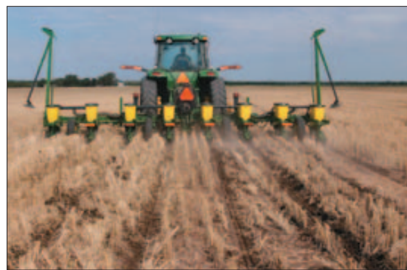
STRIP TILL AND PLANT: Some producers are finding that strip tilling and planting in one field operation fits them best. The fieldwork can be done in one operation saving time, fuel and labor, while conserving limited moisture.
