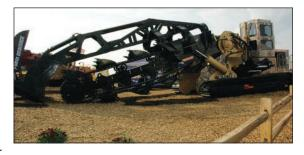
is designed for professional contractors working with water mains. It has a digging depth of 14 feet and width of 60 inches. Contact Tesmec, Alvarado, Texas, at 800-851-5102 or tesmec.com.
