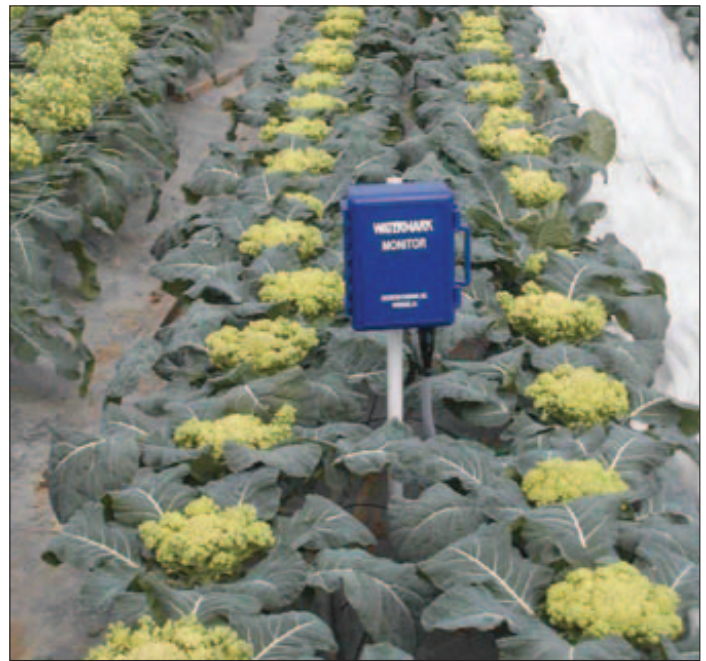
DATA LOGGER: A moisture monitor is a data logger that activates records and saves Watermark soil moisture reading until the grower can download data.
