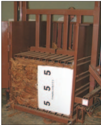
Big balers compress tobacco into a 500- to 600-pound package, measuring 42 inches by 42 inches by 40 inches.
