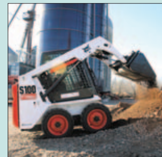
BOBCAT S100: Bobcat is replacing its 533 skid-steer loader with the new S100 model, which is rated at 1,000-pounds capacity and measures only 50 inches wide for tight maneuvering. The S100 is powered with a four-cylinder, 33.5-hp diesel engine.
