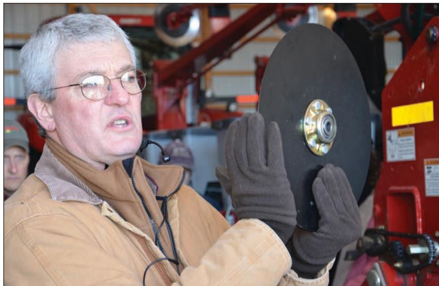
**CHECK WEAR:** Barry Fisher suggests measuring the wear of disk openers on planters vs. new openers, no matter which color of planter you operate.
