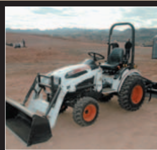
CT120: The 120 offers a tight 89-inch turning radius and a working width of less than 4 feet. The 20-hp model is available with a variety of attachments.
