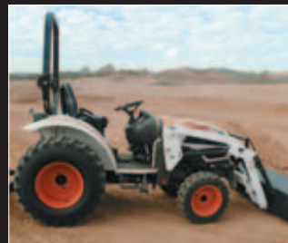
CT225: The new 27-hp CT225 compact tractor features a three-range hydrostatic transmission.
