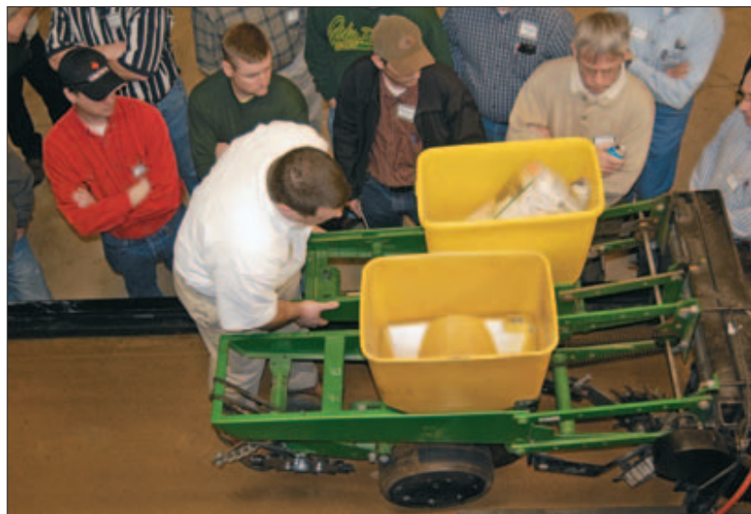
PLANTER PREP: Wiggle the planter row units to make sure they are level and the bushings are tight.
