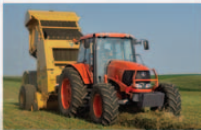
M135X — Intelli-Shift™ transmission, added power and torque with an electronic common rail fuel system for less noise and enhanced fuel efficiency.
