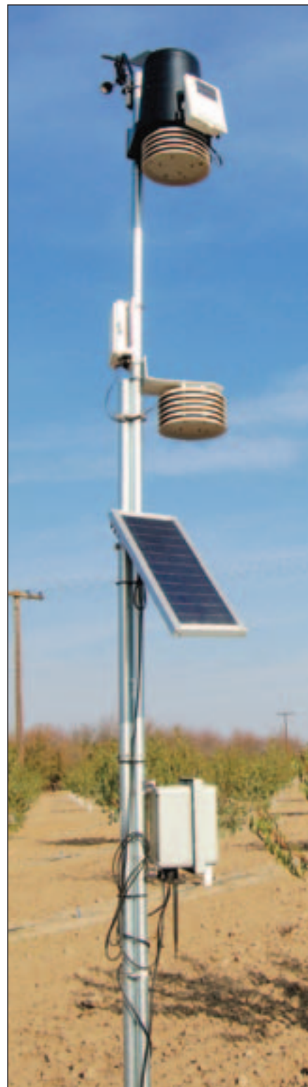
FIELD SCRUTINIZER: PureSense monitors the temperature and humidity above and within the canopy.
