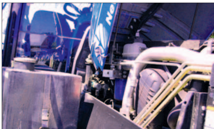
TWIN-FUELED: This Elsbett auxiliary fuel tank feeds diesel fuel to fuel injectors until the engine automatically switches to straight vegetable oil.
