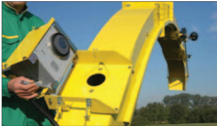
MOISTURE MONITORING: HarvestLab brings on-the-run tracking of silage moisture to forage choppers.
