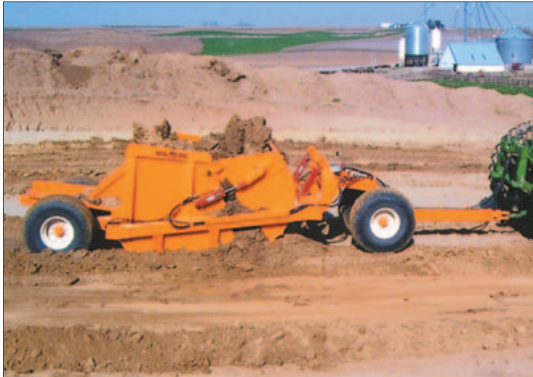
A BIGGER BIG DOG: The new 11-yard forced-ejection scraper from Big Dog adds beef to a line of well-known smaller models. The new machine is sized for 160- to 240-hp tractors.
