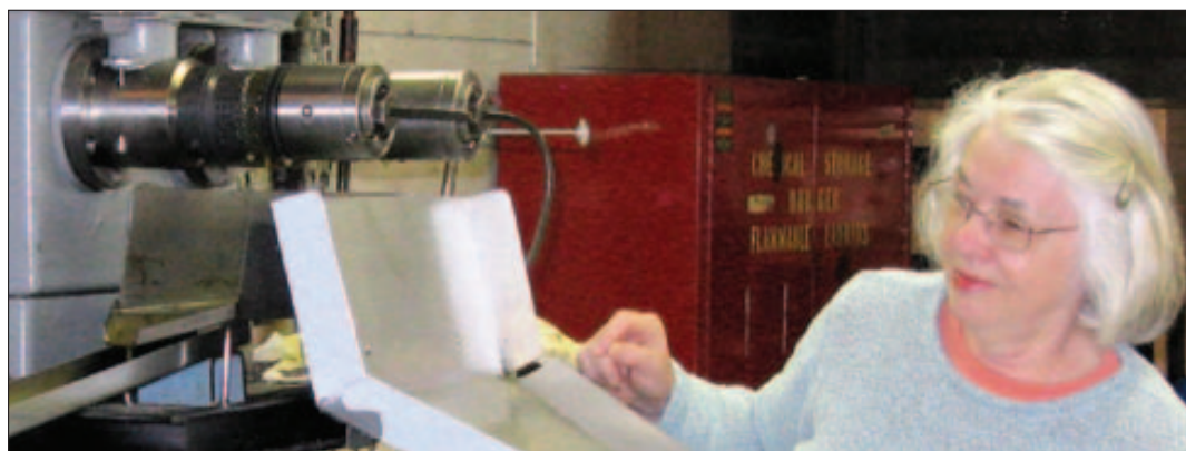
FUEL OIL: An expeller squeezes out oil on one side and meal on the other. Mary Carol Frier is expected to return to Ag Progress Days with the oilseed press demonstration.
