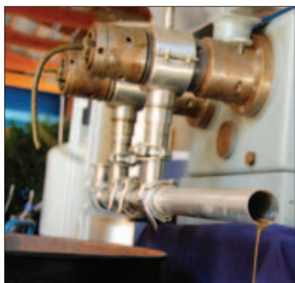
FUEL OIL: An expeller squeezes out oil on one side and meal on the other. Mary Carol Frier is expected to return to Ag Progress Days with the oilseed press demonstration.
