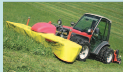
GROUND-HUGGING: Terratrak TT270 is a low-slung tractor with lots of hydraulic power. The Swiss-made machine is powered by a four-cylinder turbocharged Detroit Diesel.
